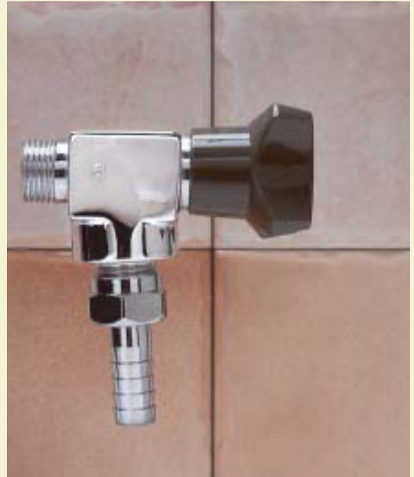
Built-in backflow protector. O-ring sealing and Teflon coated disc against adhesion.
